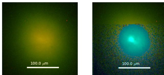
**Figure 1:** Real-colour images of thermalised photons in our dye-filled microcavity. Left: just below threshold. Right: just above threshold, showing macroscopic occupation of the lowest energy state.
