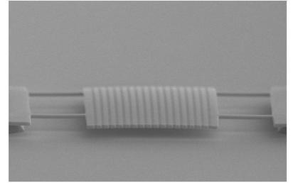
**Figure 2:** MEB view of a photonic crystal nanomembrane
