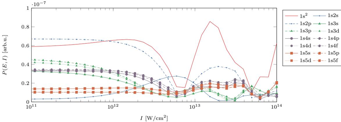
**Figure 2:** Amplitude of the different photoelectron peaks, corresponding to bound states of He I, as a function of control pulse ( $P_2$ ) intensity. The peaks are those found in the  $\beta_1$  coefficient in the Legendre decomposition of the angular photoelectron spectrum, corresponding to transitions driven with an odd number of photons.
