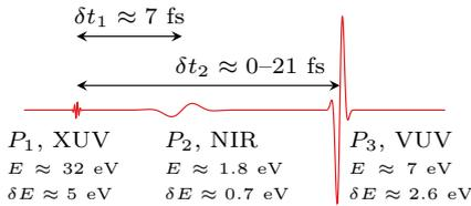
**Figure 1:** The pulse scheme:  $P_1$  is a XUV pump pulse, with broad bandwidth, capable of exciting/ionizing the atom to many bound/continuum states.  $P_2$  is a control pulse in resonance with a bound transition.  $P_3$  is a probe pulse, ionizing the remaining bound states into the continuum, where they will interfere with the states ionized by the pump pulse.
