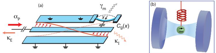
**Figure 1:** (a) A microwave resonator can be coupled capacitively to an arbitrary number of mechanical resonators. (b) Idea of introducing nonlinearity in optomechanics. Inside the cavity (blue) there is a quantum two-level system (green) which is mechanically compliant (red).
