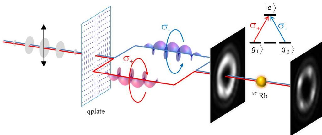
**Figure 1:** Schematic of experiment: linearly polarised probe light is converted via a qplate into light entangled in polarisation and phase structure before being transmitted through cold Rb atoms. The intensity profiles before and after interaction with the atoms are shown as insets.
