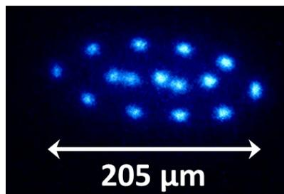
**Figure 1:** *Small  $\text{Be}^+$  Coulomb crystal obtained with axial and radial trap frequencies of  $97 \times 2\pi$  kHz and  $365 \times 2\pi$  kHz, respectively.*
