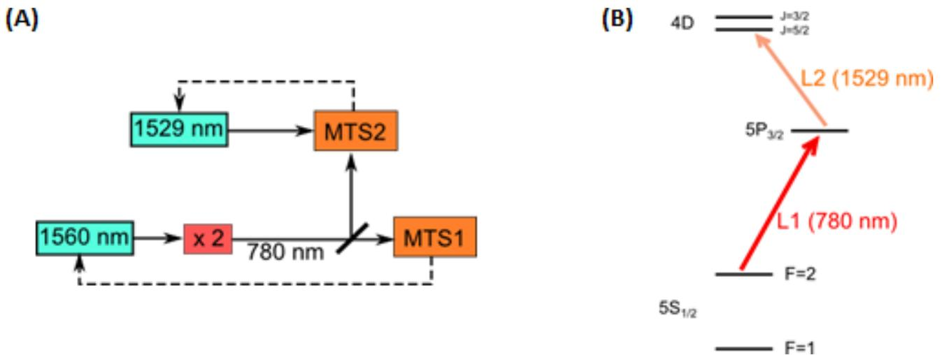
**Figure 1:** (A) Schematic depicting the laser frequency stabilization approach in our experiment. (B) Atomic transitions involved in MTS and DROP spectroscopy (see text).
