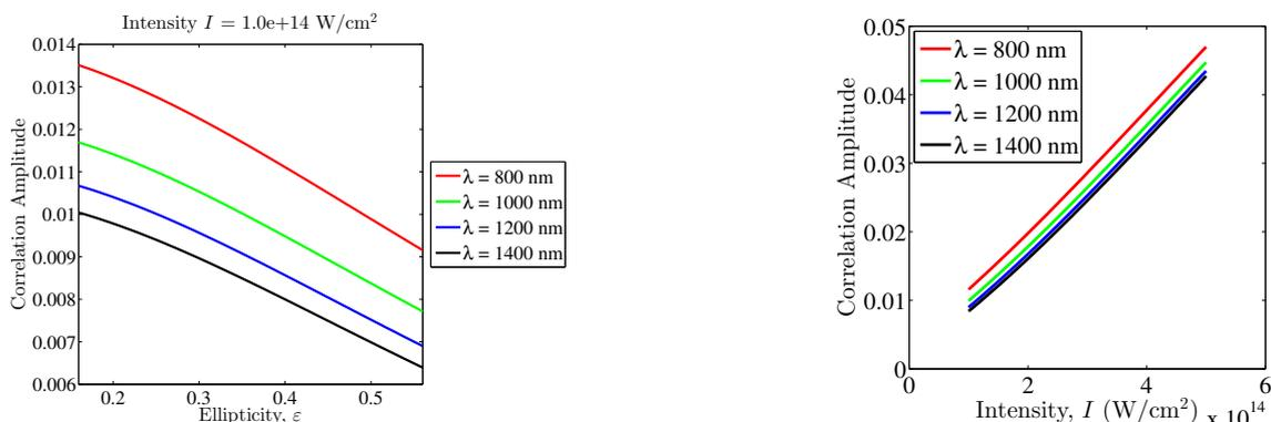
**Figure 1:** Variation of correlation amplitude with ellipticity and field strength for laser induced coupling between  $^1S$  and  $^2P_{3/2}$  state of  $Ar^+$ , that contributes to correlated sequential ionisation pathway.
