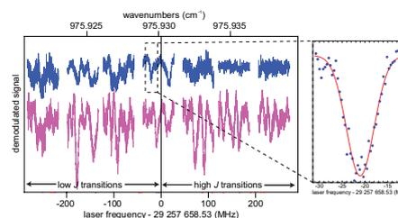
**Figure 1:** Linear absorption spectroscopy of a MTO-seeded supersonic jet, in the vicinity the R(20) CO<sub>2</sub> laser line frequency (0 MHz on the bottom axis). Lower pink curve: translational temperature  $\geq 5$  K. Upper blue curve: translational temperature  $\sim 1$  K. The inset is a zoom on a single line.
