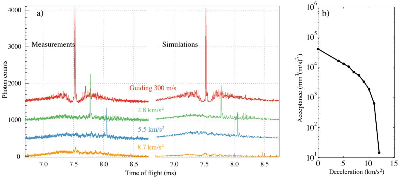
**Figure 1:** a) A time-of-flight measurement (left) compared with trajectory simulations (right) showing the deceleration of SrF molecules. b) Simulation results that illustrate the unavoidable decrease of acceptance with increasing deceleration strength. The observed deceleration matches the design efficiency.
