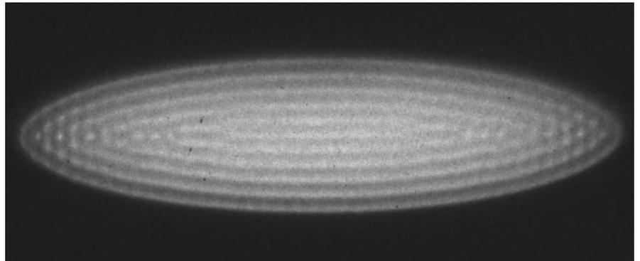
**Figure 1:** *Picture of a Coulomb crystal made of few thousands of calcium ions, laser cooled in a linear quadrupole trap*
