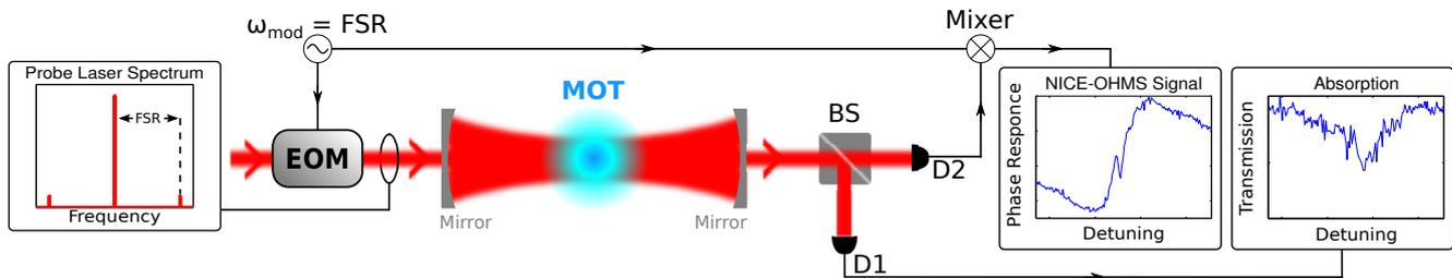
**Figure 1:** A modulated laser beam interacts with cold  $^{88}\text{Sr}$ -atoms and heterodyne detection is performed.
