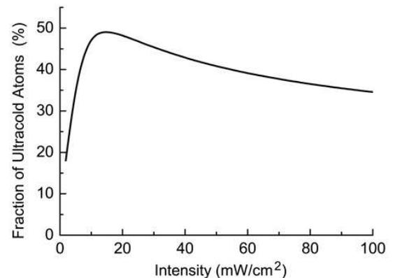
**Figure 1:** Fraction of ultracold atoms in a cold atomic cloud, detuning equals to  $-2\gamma$ .
