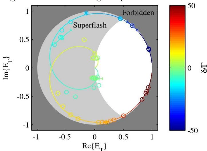
**Figure 1:** *Reconstruction, as function of the probe frequency detuning, of the transmitted field in a cold cloud with an optical density of 19. The open circles are the data points and the plain curve the theoretical prediction.*
